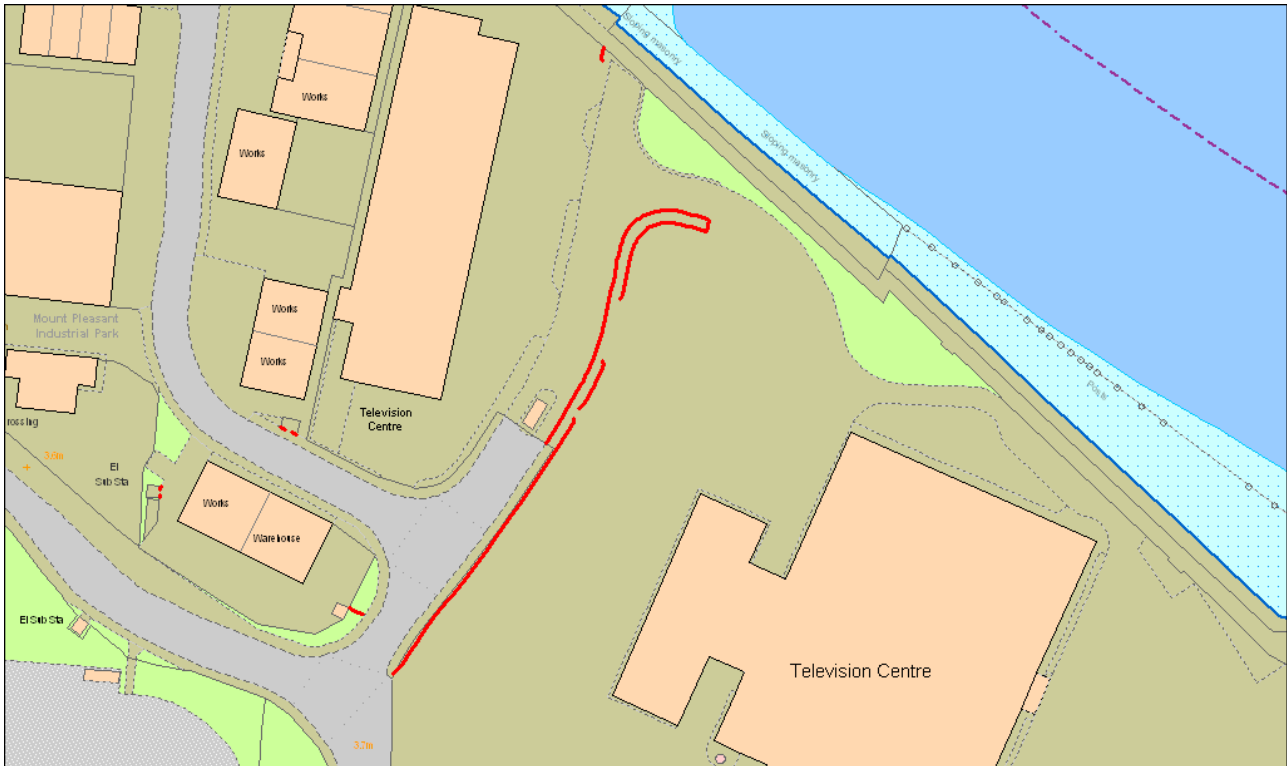
Figure 21: example of a non-bounding line (shown in red)
